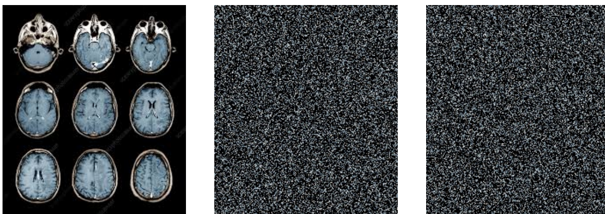
Figure 9: Decryption with a mismatched LFSR key on the Brain MRI image: (left) original, (centre) encrypted, (right) incorrectly decrypted output confirming complete key sensitivity.
