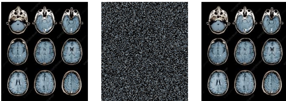
Figure 8: Ternary LFSR encryption/decryption on a Brain MRI image: (left) original, (centre) encrypted, (right) correctly decrypted using the matching LFSR key.
