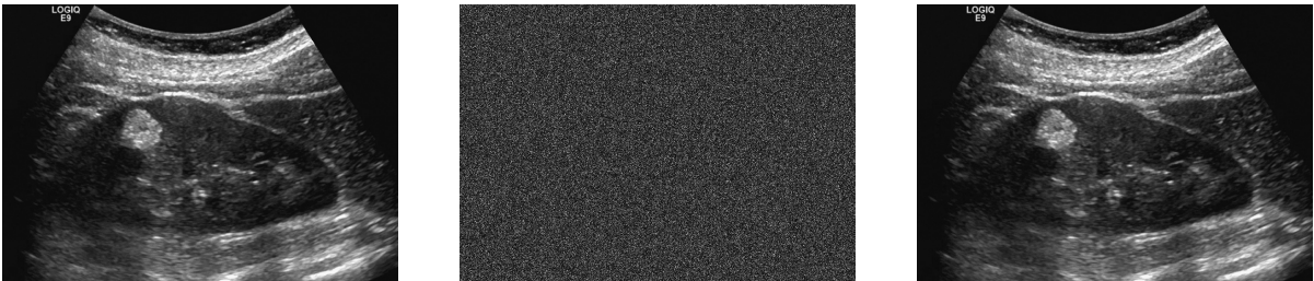
Figure 3: Ternary LFSR encryption/decryption on a Kidney Ultrasound image: (left) original, (centre) encrypted, (right) correctly decrypted using the matching LFSR key.
