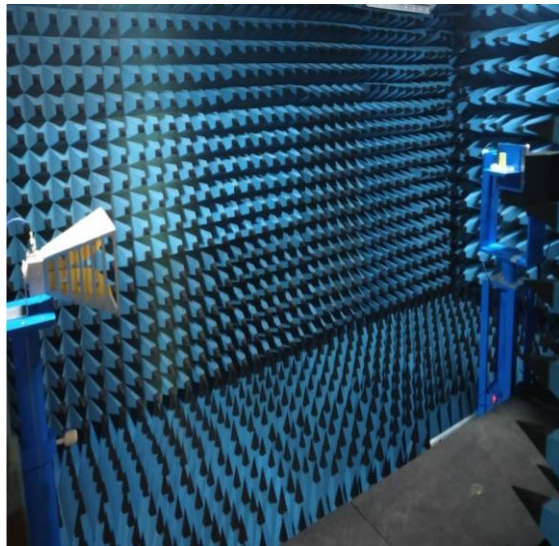
Figure. 9. Radiation pattern measurement of CPW fed quarter wave monopole antenna with ECSRR EBG reflector in Anechoic chamber
